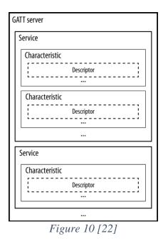
Our application has one service. This service has four characteristics. Each sensors data is
