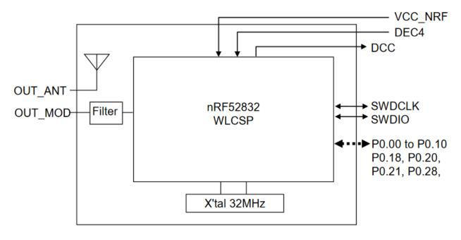
BLE Module on BLE Evaluation Board
